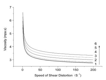
**Fig. 13.** The changes in the viscosity of pure and magnetized water with the speed of shear pure and distortion at different magnetized times.
