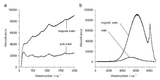
Fig. 4. The Raman spectra of magnetized water and pure water in the ranges of 20–1900 cm<sup>-1</sup> (a) and 2000–9000 cm<sup>-1</sup> (b), respectively.
