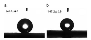
**Fig. 9.** The angles of contact of magnetized water (a) and pure water (b) on the surface of copper.
