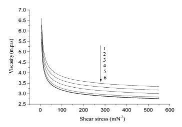
Fig. 12. The changes of the viscosity of magnetized water with the shear stress at different magnetized times.
