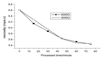
**Fig. 14.** The changes in the viscosity of magnetized water with increasing magnetized times at 3000 and 4000 G, respectively.
