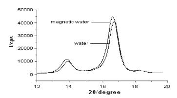
Fig. 6. Diffraction spectra of X-ray for pure and magnetized water.
