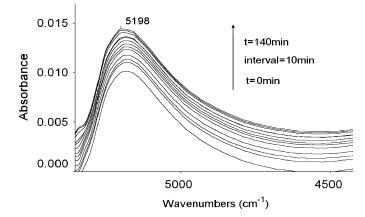
Fig. 3. Changes in the infrared absorption of water with increasing magnetized time in  $4000-6000\,\mathrm{cm}^{-1}$ .
