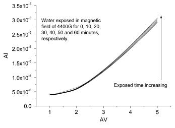
**Fig. 15.** The relationship of the electric-current strength (Al) versus voltage (AV) for magnetized water at different magnetized times of 0, 10, 20, 30, 40, 50 and 60 min.
