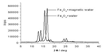
**Fig. 7.** The spectra of X-ray diffraction for the complexes of magnetized water plus nanometer  $Fe_3O_4$  and pure water plus nanometer  $Fe_3O_4$ .
