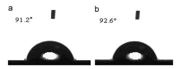
**Fig. 10.** The angles of contact of magnetized water (a) and pure water (b) on the surface of graphite.
