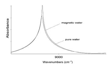
Fig. 2. The absorption spectra of magnetized and pure water in the range of  $8000-10,000\,\mathrm{cm}^{-1}$ .
