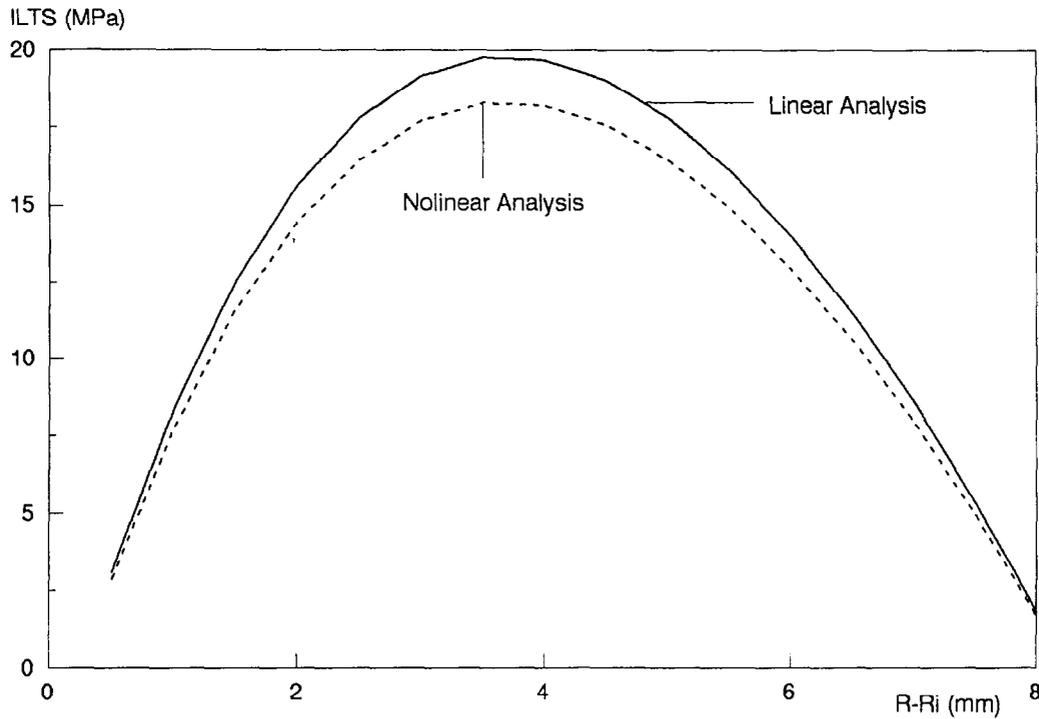
Figure 12 Effect of large deflection on ILTS distribution along the thickness
