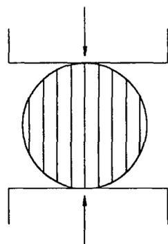
Figure 3 Diametrical compression disk specimen<sup>11</sup>
