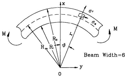
Figure 9 Uniform moment loading on curved beam
