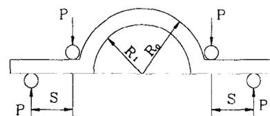
Figure 8 Four-point curved beam specimen
