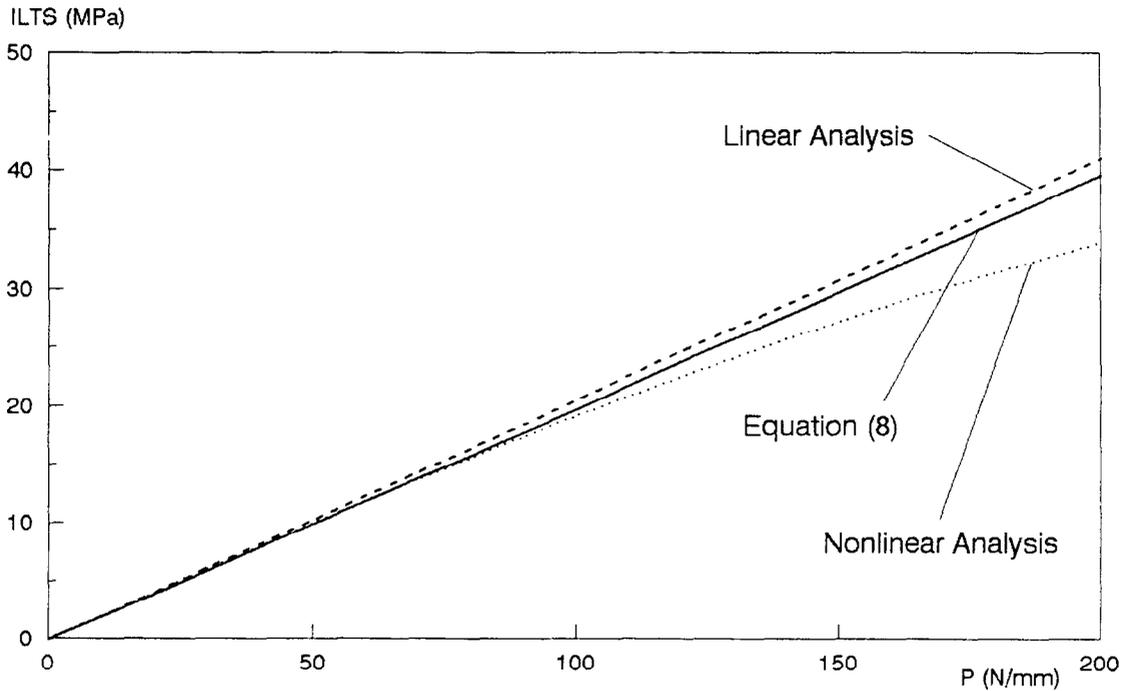
Figure 11 Effect of large deflection on maximum ILTS
