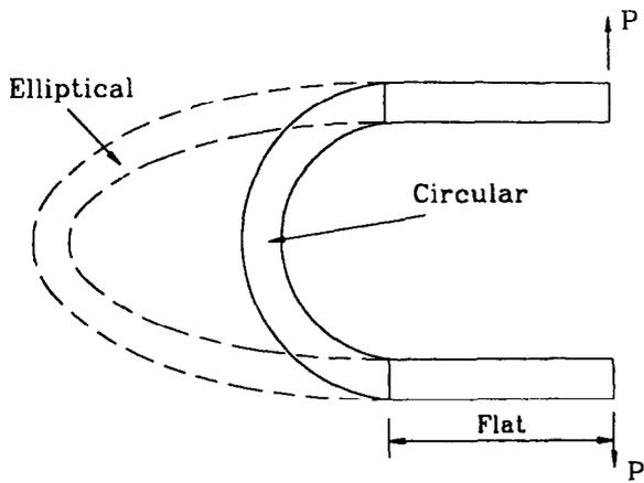
Figure 4 Semicircular or elliptical specimen<sup>13</sup>
