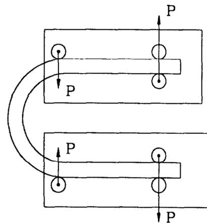
Figure 7 Pure moment on curved beam<sup>12</sup>
