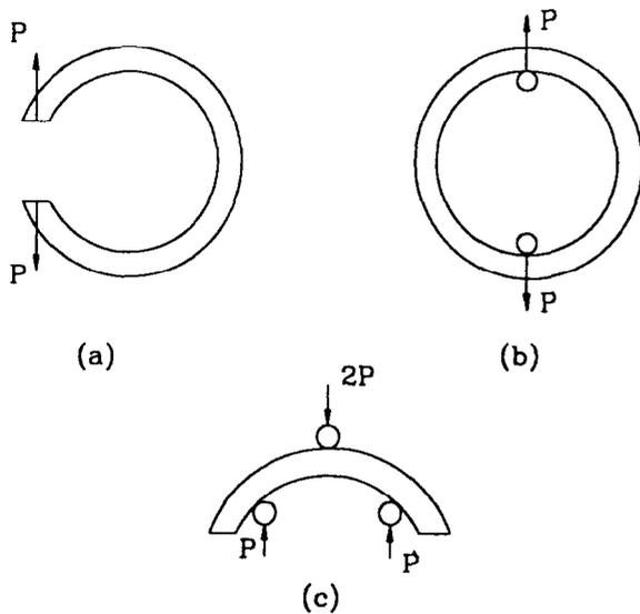
Figure 5 Ring or curved beam specimens<sup>14</sup>
