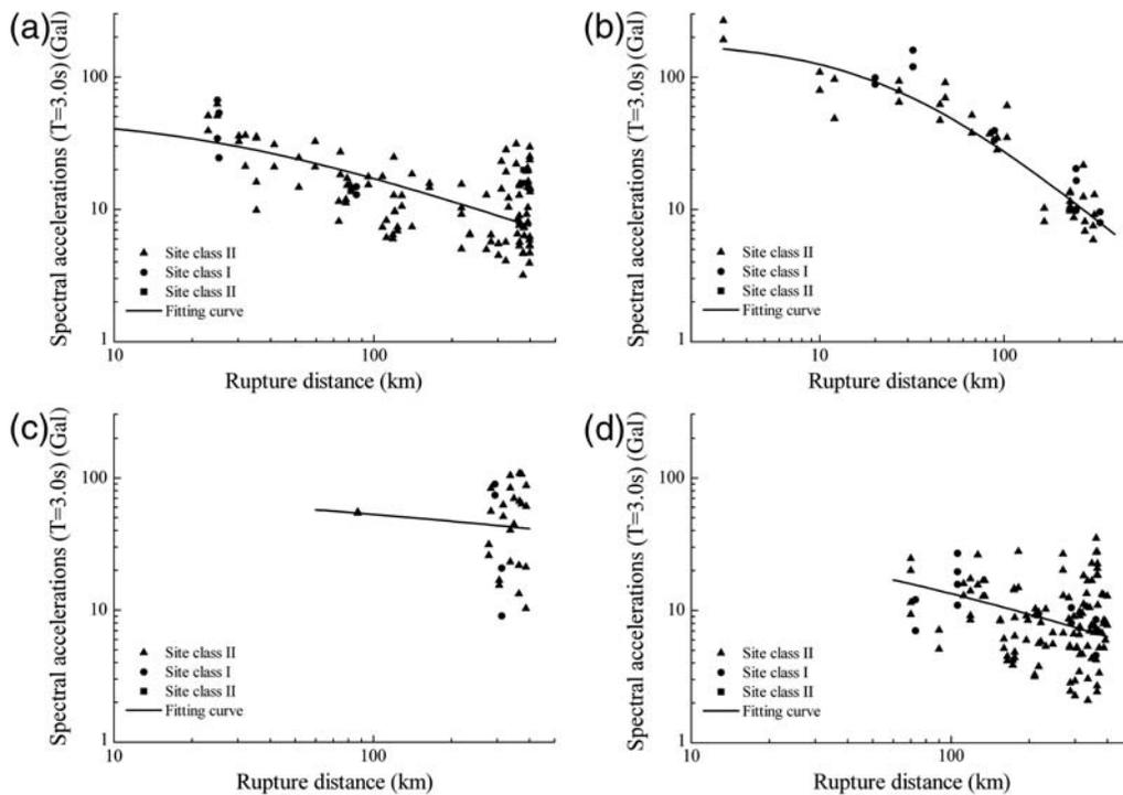
**Figure 7.** Spectral accelerations at period of 3.0 s versus rupture distance from horizontal components of the Wenchuan earthquake records in different subareas and for different site conditions, and fitting attenuation curves. (a) Hanging wall area; (b) footwall area; (c) forward directivity area; (d) backward directivity area.
