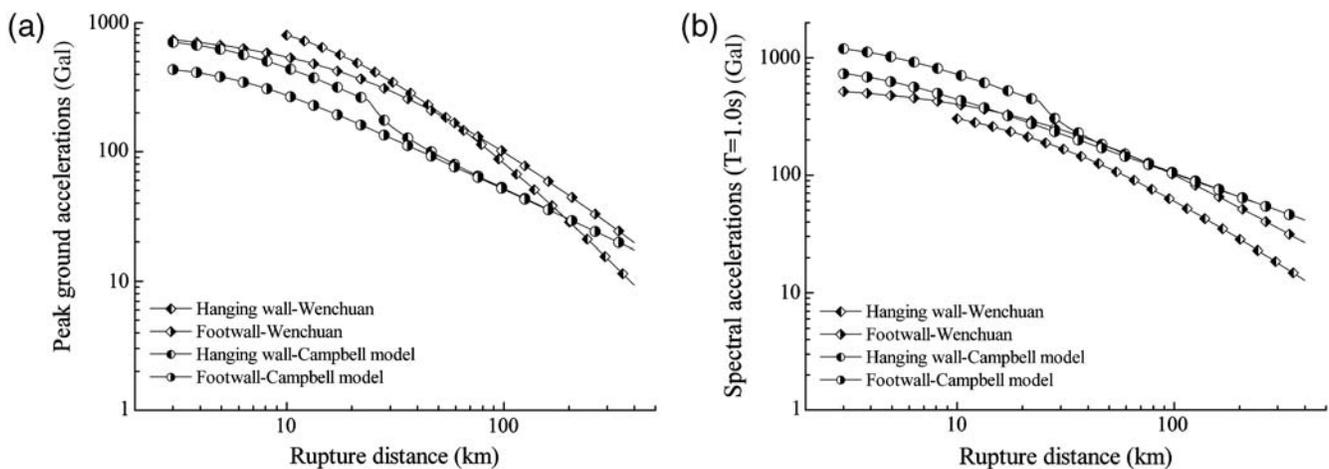
**Figure 15.** Comparison of attenuation curves of peak ground accelerations and spectral accelerations between the observed ground motions and predicted ground motions by the [Campbell and Bozorgnia \(2008\)](#) attenuation model. (a) Attenuation curves of peak ground accelerations; (b) attenuation curves of spectral accelerations at periods of 1.0 s.
