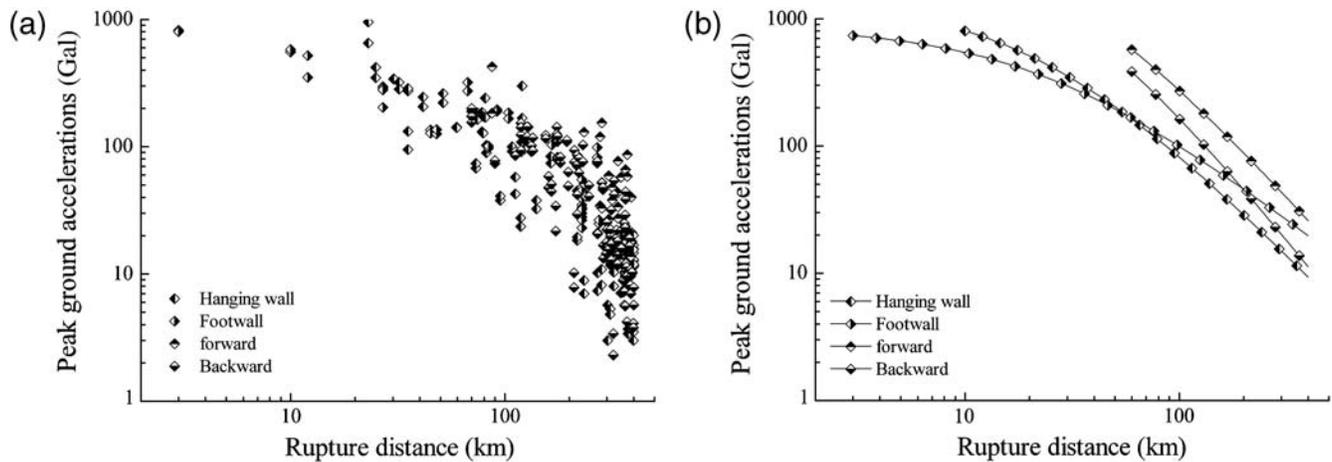
**Figure 9.** Peak ground accelerations versus rupture distance and relative fitting curves of attenuation relations for horizontal components of the Wenchuan earthquake records in different subareas and for site class II. (a) Observed data; (b) fitting curve of attenuation relations.
