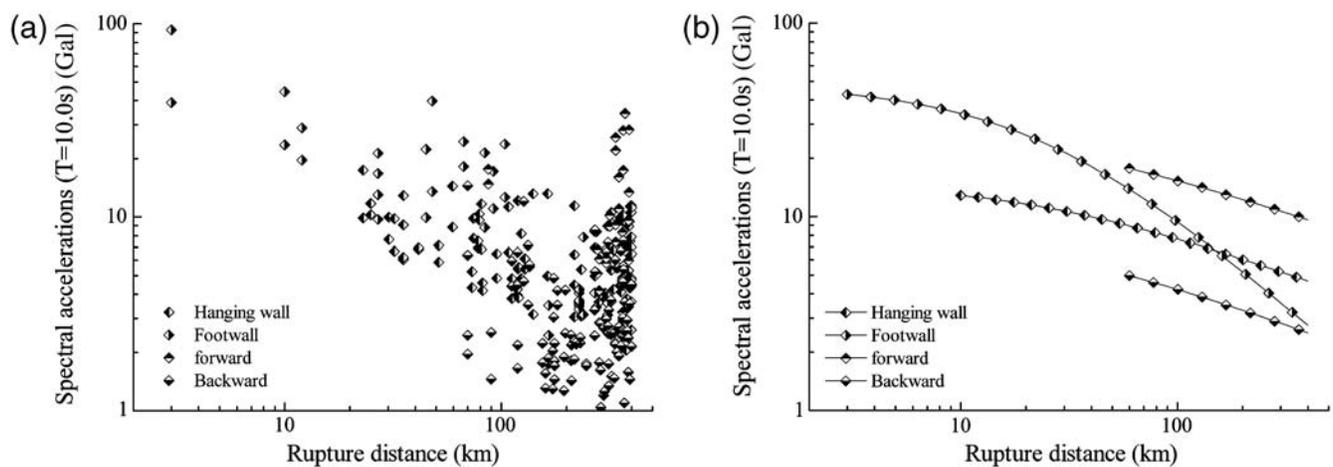
**Figure 13.** Spectral accelerations at spectral period of 10.0 s versus rupture distance and relative fitting curves of attenuation relations for horizontal components of the Wenchuan earthquake records in different subareas and for site class II. (a) Observed data; (b) fitting curve of attenuation relations.
