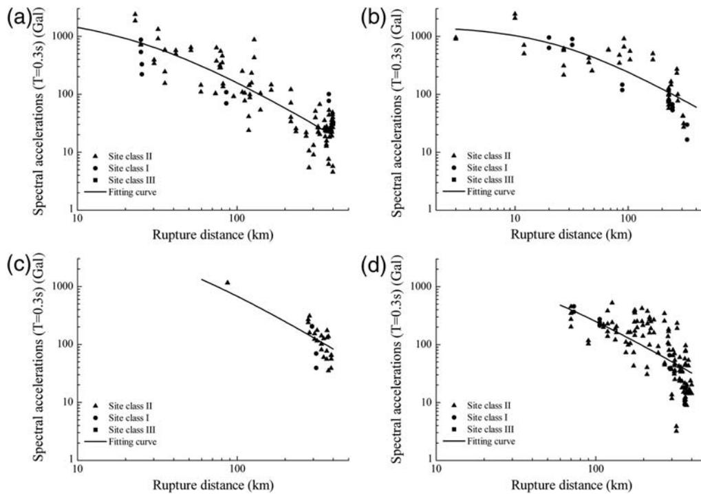
**Figure 5.** Spectral accelerations at period of 0.3 s versus rupture distance from horizontal components of the Wenchuan earthquake records in different subareas and for different site conditions, and fitting attenuation curves. (a) Hanging wall area; (b) footwall area; (c) forward directivity area; (d) backward directivity area.
