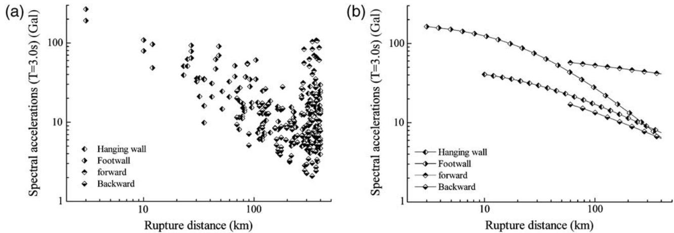
**Figure 12.** Spectral accelerations at spectral period of 3.0 s versus rupture distance and relative fitting curves of attenuation relations for horizontal components of the Wenchuan earthquake records in different subareas and for site class II. (a) Observed data; (b) fitting curve of attenuation relations.
