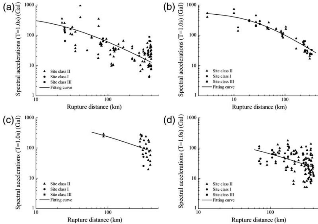
**Figure 6.** Spectral accelerations at period of 1.0 s versus rupture distance from horizontal components of the Wenchuan earthquake records in different subareas and for different site conditions, and fitting attenuation curves. (a) Hanging wall area; (b) footwall area; (c) forward directivity area; (d) backward directivity area.
