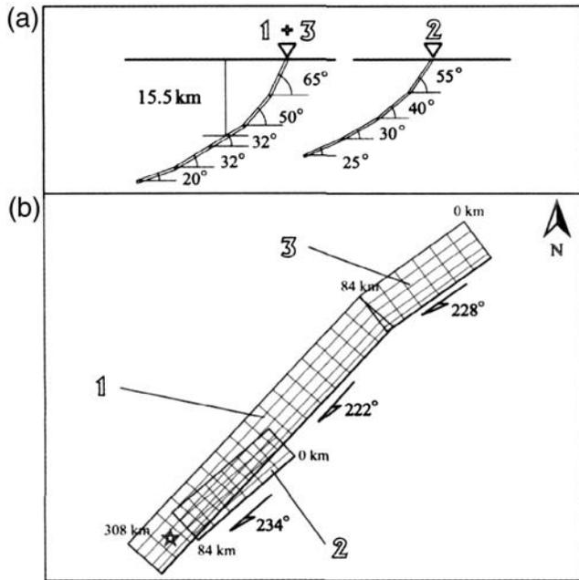
**Figure 3.** Wang’s fault model for the Wenchuan earthquake (Wang *et al.*, 2008). Model unit 1 and 3 modeling the Yingxiu–Beichuan fault, and unit 2 modeling the Guanxian–Jiangyou fault. (a) Cross section of the fault model; (b) surface projection of the fault model.
