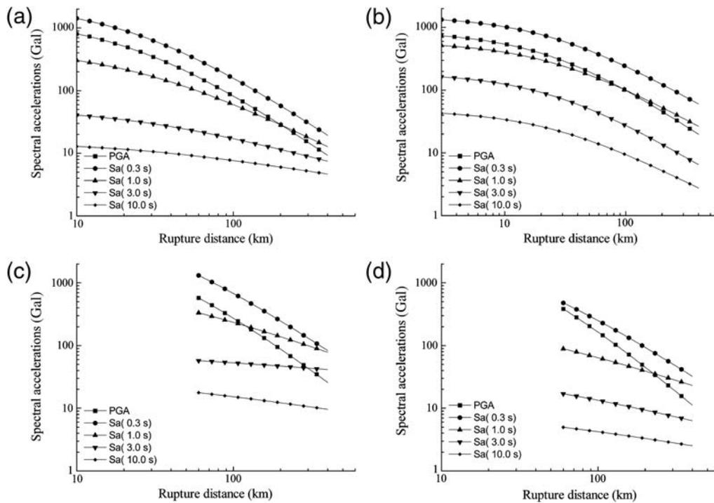
**Figure 14.** Attenuation curves of peak ground acceleration and spectral accelerations at periods of 0.3 s, 1.0 s, 3.0 s, and 10.0 s for the Wenchuan earthquake ground motions in different subareas. (a) Hanging wall area; (b) footwall area; (c) forward directivity area; (d) backward directivity area.
