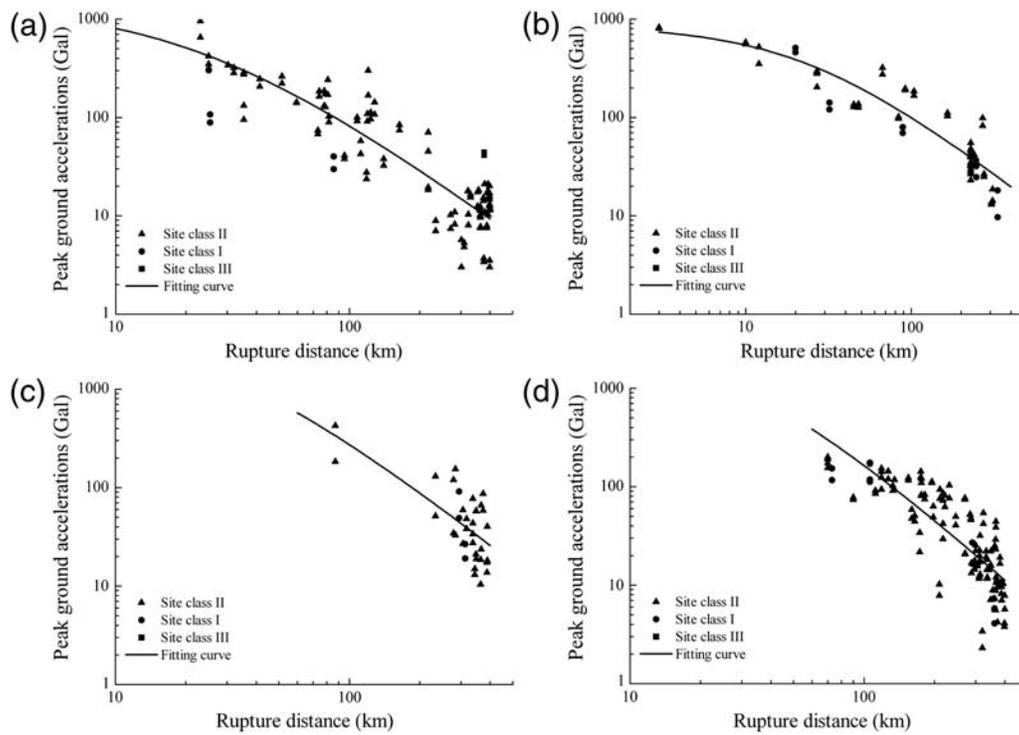
**Figure 4.** Peak ground accelerations versus rupture distance from horizontal components of the Wenchuan earthquake records in different subareas and for different site conditions, and fitting attenuation curves. (a) Hanging wall area; (b) footwall area; (c) forward directivity area; (d) backward directivity area.
