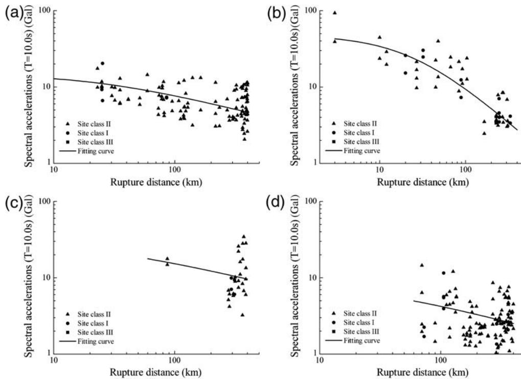
**Figure 8.** Spectral accelerations at period of 10.0 s versus rupture distance from horizontal components of the Wenchuan earthquake records in different subareas and for different site conditions, and fitting attenuation curves. (a) Hanging wall area; (b) footwall area; (c) forward directivity area; (d) backward directivity area.
