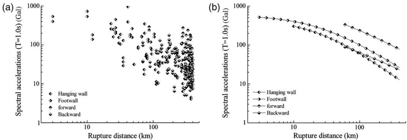
**Figure 11.** Spectral accelerations at spectral period of 1.0 s versus rupture distance and relative fitting curves of attenuation relations for horizontal components of the Wenchuan earthquake records in different subareas and for site class II.
