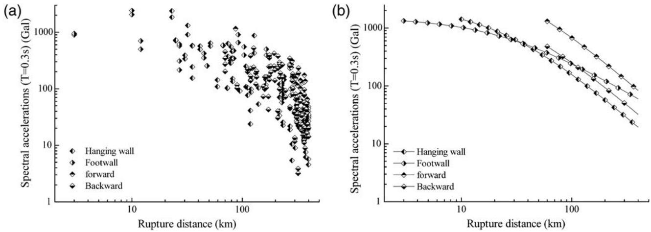
**Figure 10.** Spectral accelerations at spectral period of 0.3 s versus rupture distance and relative fitting curves of attenuation relations for horizontal components of the Wenchuan earthquake records in different subareas and for site class II. (a) Observed data; (b) fitting curve of attenuation relations.
